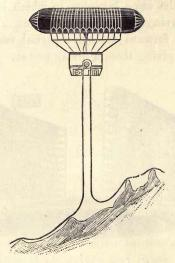
over a pulley situated in the car of the balloon. The pulley is rotated by an electro-motor in the car and thus draws the balloon along in the direction of the rope.
